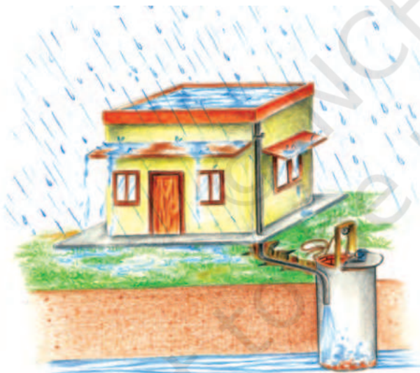
(b) Recharge through Abandoned Dugwell
